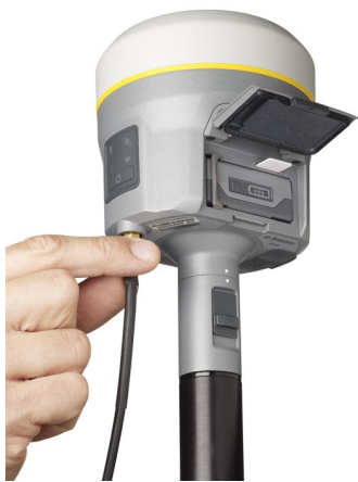
Connecting remote radio antenna cable to the receiver
