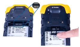
The card holder can hold two nanoSIM cards, or one nanoSIM card and one microSD card at a time. Insert your cards as needed, as follows:
