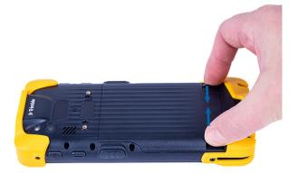
2. Push the battery forward and lift to remove it.
