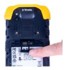
The card holder can hold two nanoSIM cards, or one nanoSIM card and one microSD card at a time. Insert your cards as needed, as follows:
