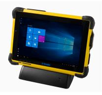
• You can charge the battery pack in the T10 tablet by connecting the AC-DC adapter directly to the DC-in port on the T10 tablet or through the DC-in port on the office dock while the T10 tablet is docked.
