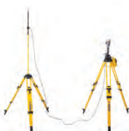
RTK base setup with remote UHF antenna
