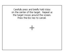
[+] (plus) sign on center and four corners completes the adjustment of touch screen.
