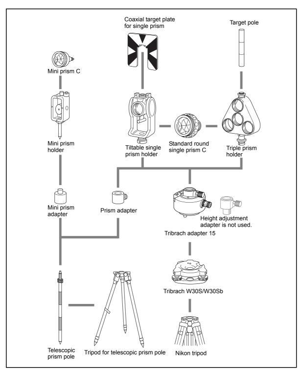
Figure 5.2 Prism reflector side
