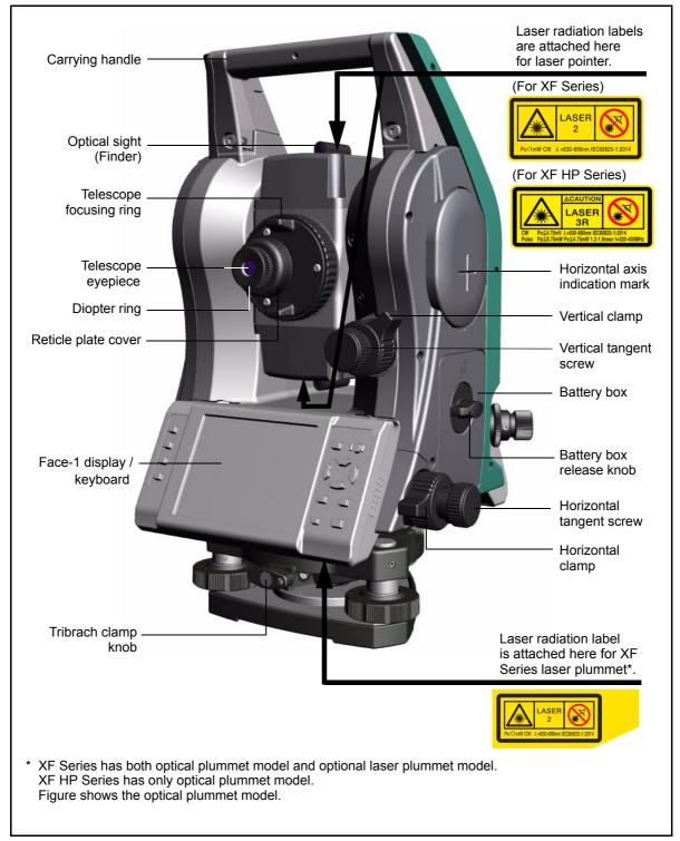
Figure 1.1 XF/XF HP Series Total Station – Face-1
