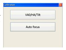
Sight a non-prism point that is between 2 m and 4 m away and focus manually using the focus ring. Then press [+] or [–] button to fine adjust the focus, once fine adjustment is complete, tap [MSR] button.
