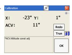
If the HA corr. setting is set to OFF, the ACH parameter is not applied to horizontal angle readings. If this setting is set to ON, both of the ACH and trunnion-axis parameters are applied to HA. If you do not complete the second step, the trunnion-axis parameter remains set to zero, and only the ACH parameter is applied. If ACV, ACH, X, or Y is out of range, OVER appears. Press any key to return to the first observation screen.
