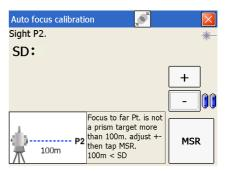
Once both the near and far measurements are complete, the calibration constant will be calculated. If the calibration is successful, the following screen will be displayed.
