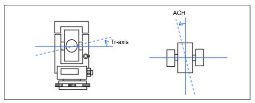
Because the amount of compensation changes according to the vertical angle, when compensation is enabled there is a slight movement in horizontal angle even if you clamp the tangent screw.
