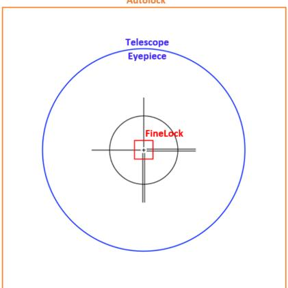
From the table above you can see that when using FineLock technology, to have an undisturbed measurement, the second prism needs to be outside of the 0.16 gon field of view. Defining the minimum offset as an angle is not practical for a user in the field, so instead, a minimum offset delta (as an offset or height difference) is used instead. This is the minimum delta required between the primary prism and other prisms, to ensure that the sighting to the desired prism is not influenced.
