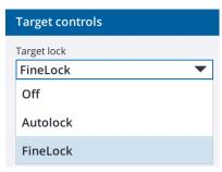
Instrument functions will show which mode the tracker is set to. Tap and hold on the Autolock/FineLock button in instrument functions will provide a shortcut to the target controls form.
