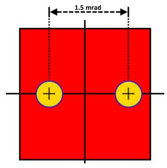
So typically, the 1.5 mrad target distance is still not sufficient. A sufficient target separation is reached with an angle difference of 2.75 mrad which is slightly larger than the size of the FineLock receiver diode. However, this is still assuming that the two targets are at a very similar distance, which is often not going to be the case.
