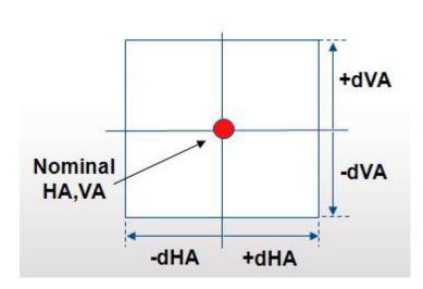
Using the parameters of the tolerance window, you can define how much the instrument may turn left/right or up/down. If the FineLock technology turns to a target and in doing so exceeds one or both of the tolerance window limits, it automatically turns back to the starting position.
