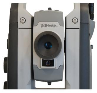
When using the FineLock lens aperture you need to ensure that you enable the corresponding option in the Trimble Access software. In General survey enable the "Using FineLock lens aperture" checkbox under *General Survey > Instrument > Target controls*
