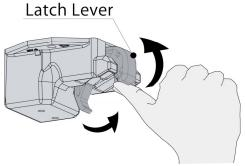
If the Latch lever is locked, please check if the Balancing Sensors are seated properly. \*You will see 2 metal dots through the holes on housing. Those are the Balancing Sensors.
