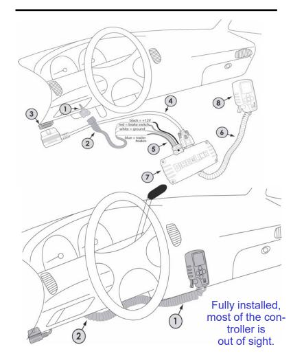
The required electrical connections are indicated by the numbers in the diagram above:
