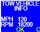
The **TOW VEHICLE INFO** screen displays **MPH** and **RPM** those two parameters from the tow vehicle's network. The only time engine RPM is displayed is when velocity is zero. As soon as velocity is detected the engine RPM value disappears and only MPH is displayed. This screen is also used to indicate successful network communication between the DirecLink and the tow vehicle.
