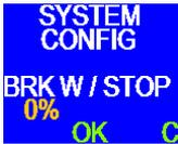
The Brake Level w/Stopped screen allows the driver to set a desired percentage level of trailer brakes to be applied when the tow vehicle-trailer is at a stop. The level can be set from 0% to 30%. When activated, the DirecLink adjusts the trailer brakes up to the setting when tow vehicle-trailer velocity is zero. This feature is helpful when stopping on steep grades or on slippery boat ramps. By having the trailer brakes applied when stopped it helps keep the tow vehicle and trailer stationary.
