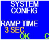
The RAMP TIME screen allows the driver to set a desired time for the controller applies power to the trailer brakes based on a time-based circuitry. The RAMP time is from ZERO (0) to FIVE (5) seconds. ZERO (0) is NO time-based control. This RAMP TIME only works when the OBD communication is failed.
