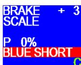
This screen indicates that the blue wire trailer brake voltage or signal wire of the four wire Delphi connector (connector #4 as outlined on page 1 of this manual) is shorted to ground. This fault completely disables your trailer brake system.
