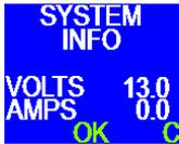
The **SYSTEM INFO** screen displays the vehicle battery voltage monitored from the black wire of the Delphi harness and the amperage output of the controller to the "blue wire" during normal braking or running the manual override.
