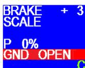
This screen indicates that the white wire [ground (-)] of the four wire Delphi connector (connector #4 as outlined on page 1 of this manual) is either not connected properly or has an intermittent connection. This wire is to be connected to the negative terminal of the tow vehicle battery only. This fault completely disables your trailer brake system.
