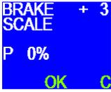
The **Brake Scale** number represents the level of trailer braking that the DirecLink will apply to the trailer brakes when the tow-vehicle brakes are applied. The value can be adjusted from +0 to +20 with +1 being very light braking and +20 being very heavy braking. (The default level is set at +3.)
