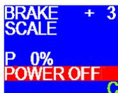
This screen indicates that the black wire (12V +) of the four wire Delphi connector (connector #4 as outlined on page 1 of this manual) is either not connected properly, has an intermittent connection or there is no power from the vehicle electrical system. This fault completely disables your trailer brake system.
