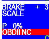
This screen indicates that the connection between the DirecLink and the OBDII connector is loose or disconnected. These are connections 3 with 4 or connections 4 with 7 as outlined on page 3 of this manual. Tightening or reconnecting the cables should resolve this problem. This fault results in the DirecLink operating in emergency mode as indicated by a "red" braking bar while vehicle braking.
