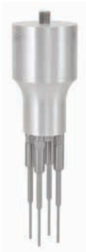
The 4 Tip Horn enables 4 samples to be processed simultaneously. This horn offers high intensity and is effective for cell disruption, mixing, homogenization and many other applications. Tip Diameter is 1/8" and the space between each tip is 1.05".
