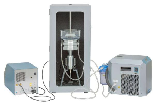
Check to ensure the O-rings and collars are seated level on the horn. The collars should not be on an angle. Check for leaks when you fill the water reservoir for the first time. Be careful not to allow water to drip into the Converter.
