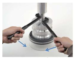
Remove the microplate horn from the converter
