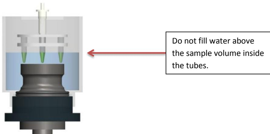
7. Turn the chiller on and set the desired temperature with the key pad. The temperature can be set as low as 4°C. *Note: Do not operate the chiller without water in the cup.* Begin to recirculate cool water through the cup horn reservoir. As the tubing fills the water level in the cup will drop. Add additional water with a pipet if necessary to ensure that the water level is the same as the sample liquid level in the tubes as indicated above.
