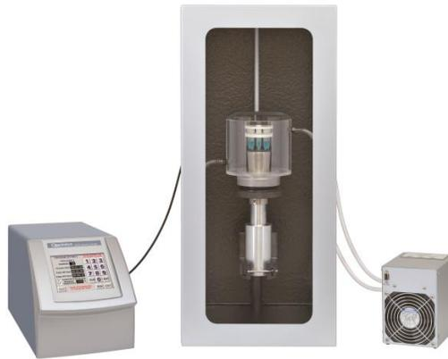
6. Using 4°C DI water, slowly add water along the side of the cup until the water level is equal to the sample liquid level inside of the sample tube (see the image below). Once the appropriate water level is determined for your sample volume and sample tubes, laboratory tape can be used to mark the water fill level on the outside of the cup. *The water level must remain constant to prevent variability when processing samples.*
