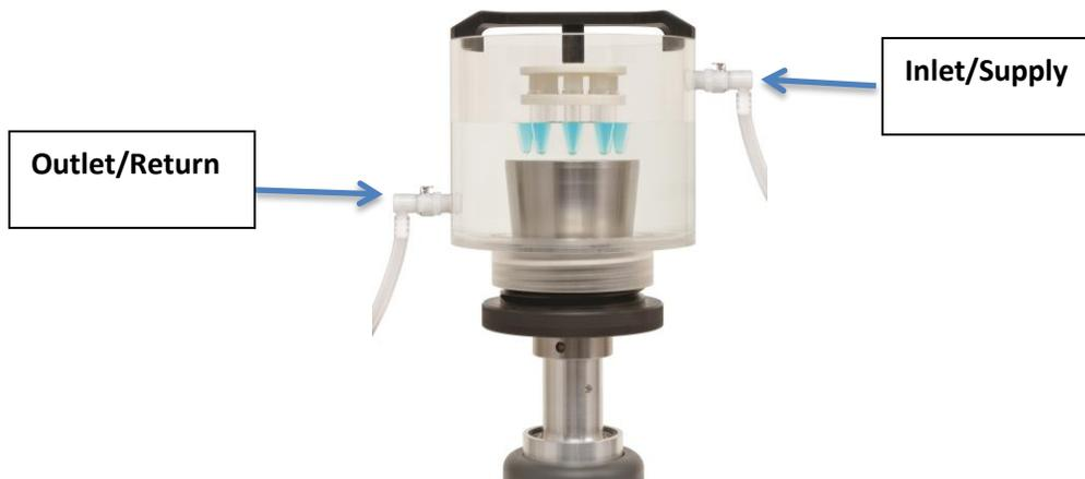
5. When using the Sound Enclosure, there are capped ports on either side. Remove the caps and pass the tubing through each port before attaching the connectors. You have the option of using the ports on either side of the enclosure.
