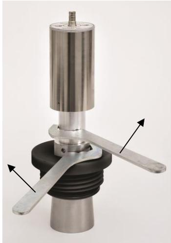
Removing the cup horn from the converter
