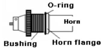
4. Hand tighten the cup horn to the converter. Then place the converter and horn assembly horn side down on a bench top. Use wrench set provided with your Sonicator to tighten the cup horn onto the converter as show in the figure below. The cup horn will malfunction if not tightened well.
