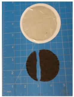
Figure 5: A sheet of buckypaper that was fractured while separating from the filtration membrane
