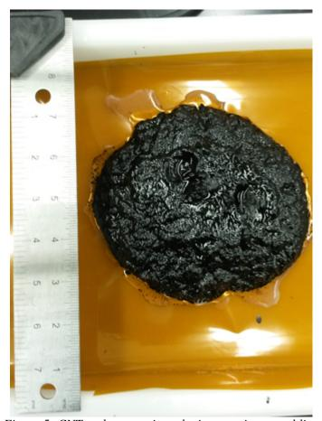
Figure 5: CNT and wax sonicated mixture prior to molding
