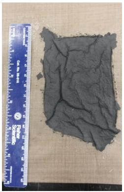
Figure 10: Sonicated sample after the vacuum bagging process
