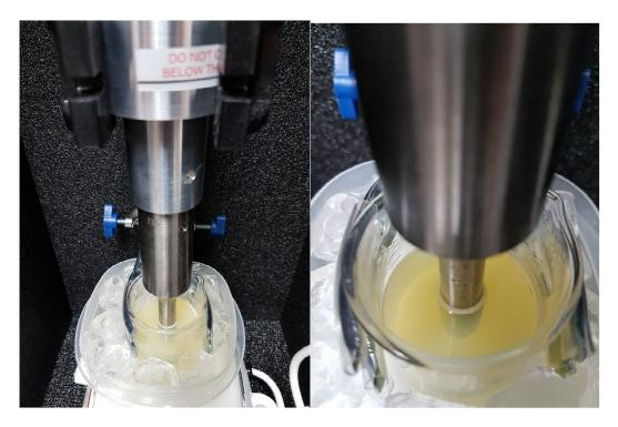
11. Once the emulsion has reached a sufficiently low particle size or level of translucence the processing may stop. The final emulsion should be clear, translucent with no surface oil observed. The nanoemulsion below is one that is produced using Axiomm Technologies' <u>µGOO</u>.
