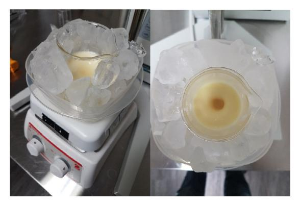
8. Turn off the stirrer and insert the ultrasonic probe into the emulsion.
