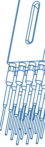
**TIP TO TIP SPACING** IS .850 INCHES (22MM)
