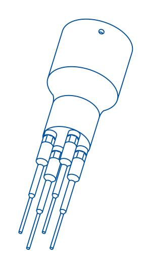
TIP TO TIP SPACING IS 1.050 INCHES (27MM)
