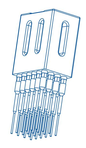
TIP TO TIP SPACING IS .708 INCHES (18MM)
