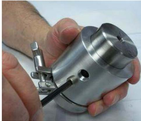
3. Tighten the plug into the floccell outlet port.
