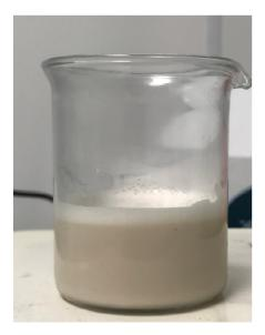
Overhead Homogenization to Form Microemulsion
