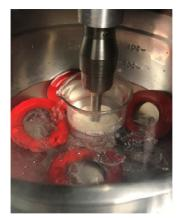
Sample secured in ice bath using flask weights
