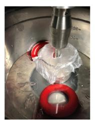
Sample secured in ice bath using flask weights with optional cover
