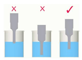
Probe submersion depth example
