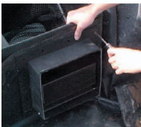
Be sure to use a large bead of silicone around opening. Hold face plate in place and line up holes with an awl.
