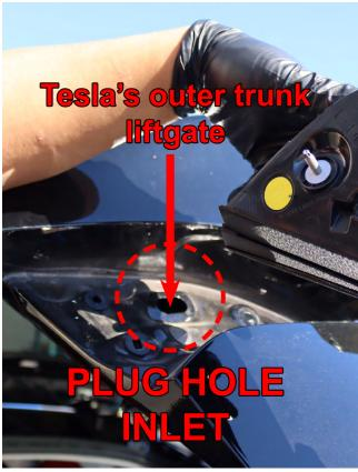
Now that you have trimmed the plug, it can be inserted easily into the outer trunk liftgate's plug hole inlet. *Please follow the same steps for the other side of the tail light's plug. Thank you!*
