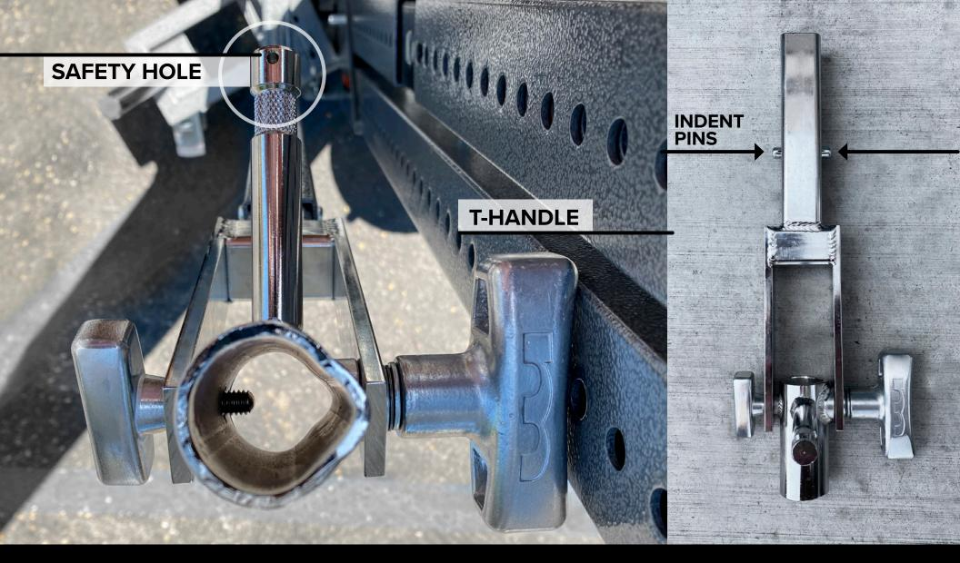
Check the combination junior / baby tip and confirm the tip has the proper locking tee handle for the junior receiver and that the baby pin saftey hole is clear and can receive a saftey cotter pin.
