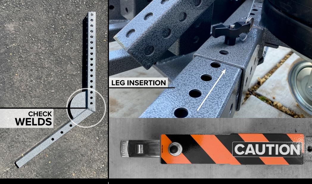
Confirm the offset arm is available and look for any bent parts or cracked welds.
