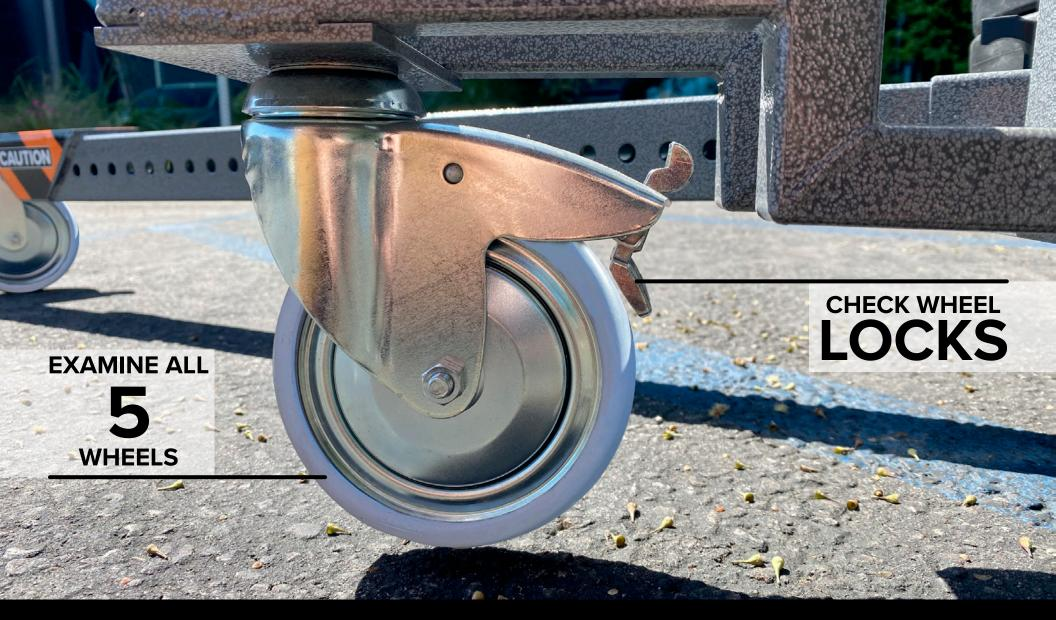
When first deploying Max a quick walk around should be performed on a daily basis.
