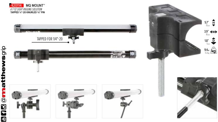
The MQ Clamp was designed to securely clamp any length T-12 light fixture without the possibility of crushing the tube. The clamp terminates to an industry standard  $\frac{3}{3}$ " pin which can be used with any  $\frac{2}{2}$ " grip head, Matthews mini or microgrip head. The  $\frac{3}{3}$ " pin is knurled to prevent unwanted rotation and is internally tapped  $\frac{4}{20}$ " to expand its rigging capabilities.
