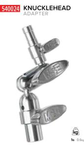
Mounts to 5%" male or 1-1%" female, and is internally threaded 3/8"-16 to support standard camera accessories. It rotates in all axis and will easily support up to 15 pounds. Made for Dots, Fingers and small light fixtures accepting 5%" male.
