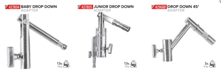
Drop Downs are most commonly used on Lighting Booms. The pivoting mount allows the use of a light box or other lighting instruments to maintain a horizontal position regardless of the angle of the boom. The 45° Angle Drop Down is primarily used with reflectors to allow their use at lower angles than most stands permit.
