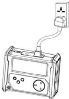
If the socket outlet is correct this will be indicated as LN,LE,NE ok PASS
