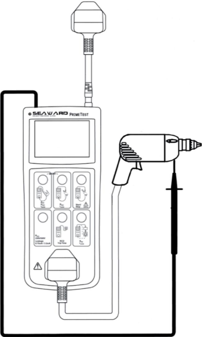
Figure 6. Testing CLII appliances, mains leakage
