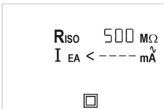
**Note: The power switch on the appliance under must be in the ON position to perform an insulation test. If no appliance is detected the PrimeTest 250 will display the following.**
