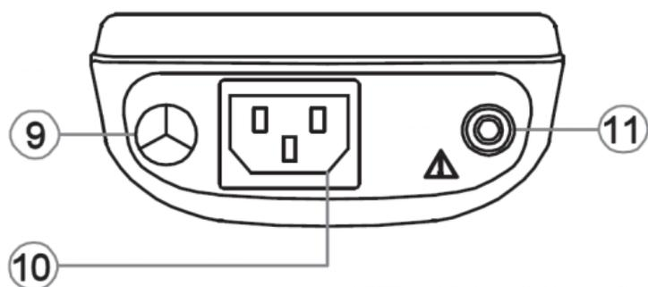
Figure 2. PrimeTest 250 End View
