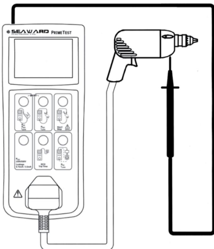
Figure 4. Testing CLII appliances, no mains leakage
