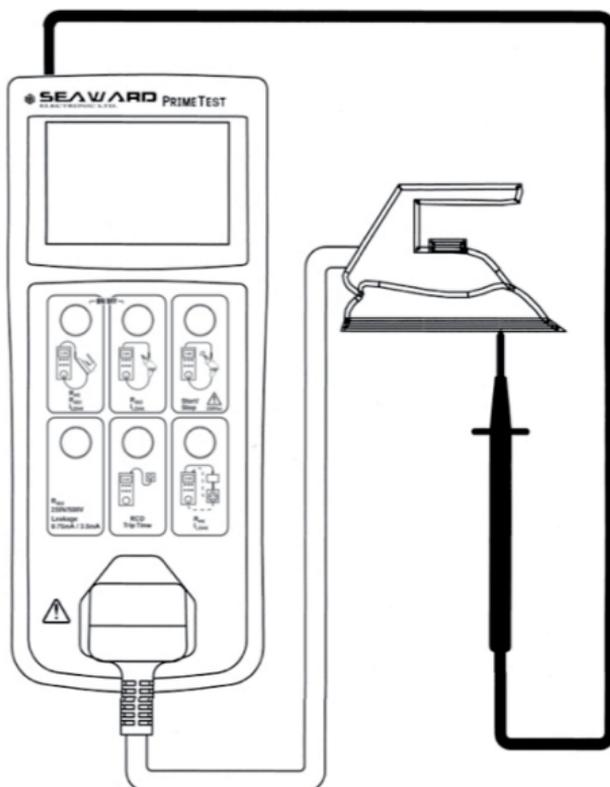
Figure 3. Testing CLI appliances, no mains leakage
