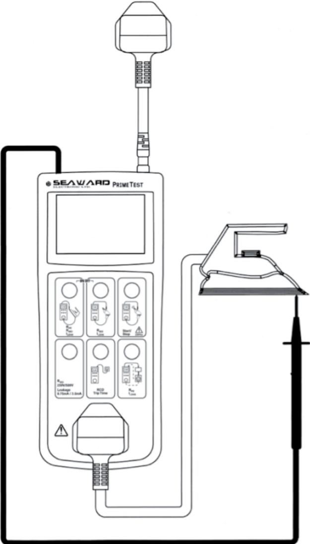
Figure 5. Testing CLI appliances, mains leakage
