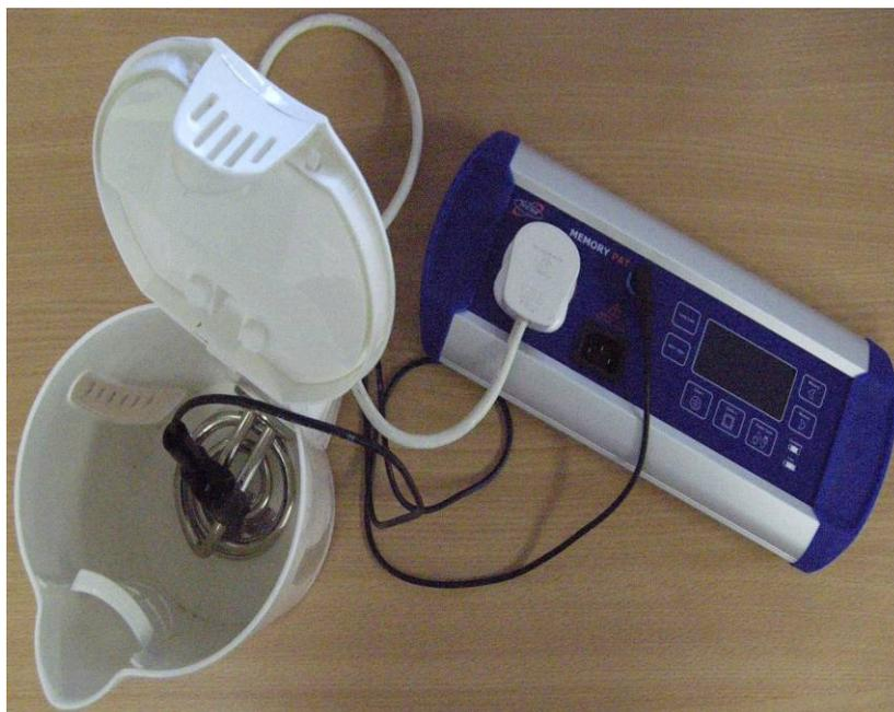
Press the Class I button. The MemoryPAT will first check that the power switch on the item is in the ON position.
