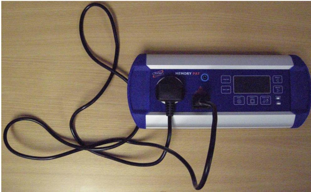
For IEC leads up to 1 metre in length, press the Power cord button. The MemoryPAT run through the tests and the results for Insulation Resistance, Earth Continuity, and Wiring will be displayed as well an overall Pass or Fail as shown below.
