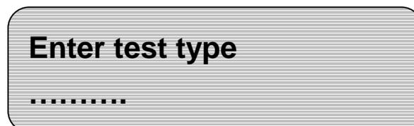
Enter the IEC lead test code and press the YES key
