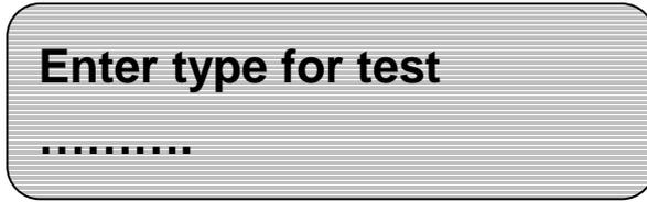
Enter the required test code that you will use to call up this test in AUTO Mode, and press YES to continue. If you enter an existing user test type it will be erased and replaced by the test you have just set up, be careful! If required it is possible to overwrite the pre-programmed test types within the tester.
