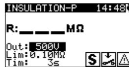
*Figure 5.12: Insulation resistance - P menu*
