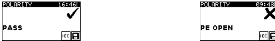
Figure 5.26: Examples of polarity test result
