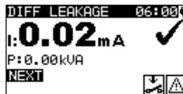
**Figure 6.11:** VDE Organizer – Differential leakage result screen
