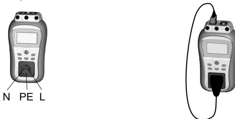
**Figure 5.25:** Polarity test of IEC cord
