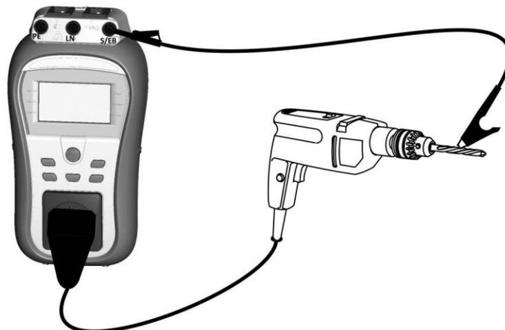
*Figure 5.13: Measurement of Insulation resistance - P*
