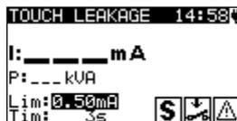
**Figure 6.17:** VDE Organizer – Touch leakage starting screen
