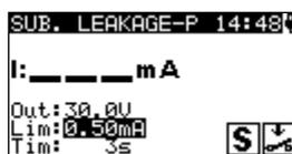
**Figure 6.37:** Substitute leakage - P starting screen
