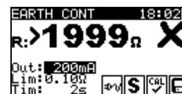
*Figure 5.7: Examples of Earth continuity resistance measurement results*
