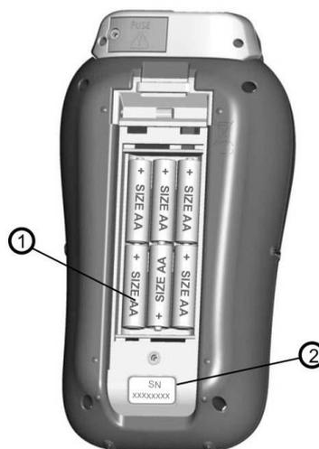
**Figure 2.4: Battery compartment**
