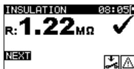
**Figure 6.30:** Insulation result screen
