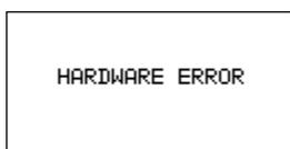
The instrument detects a serious failure. Switch OFF the instrument. Disconnect all cables and leads. Switch ON the instrument again. **Return the instrument to the repair centre if the message is displayed again.**
