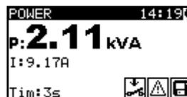
**Figure 5.40:** Example of apparent power measurement result
