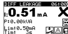
**Figure 5.29:** Examples of differential leakage current measurement result
