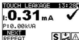
**Figure 6.40:** Touch leakage result screen
