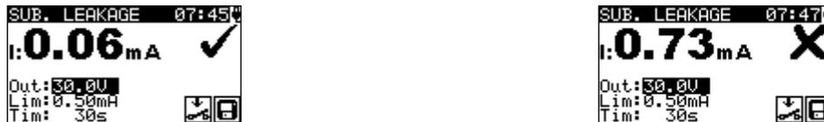
**Figure 5.19:** Example of substitute leakage current measurement results
