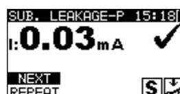
**Figure 6.16:** VDE Organizer – Substitute leakage - P result screen
