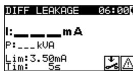
**Figure 6.10:** VDE Organizer – Differential leakage starting screen
