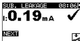
**Figure 6.32:** Substitute leakage result screen
