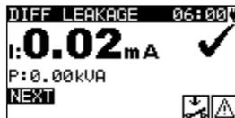
**Figure 6.34:** Differential leakage result screen
