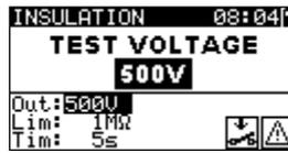
Figure 6.5: VDE Organizer – Insulation resistance starting screen
