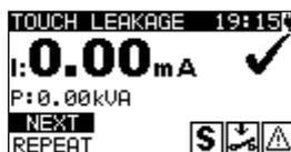
**Figure 6.18:** VDE Organizer – Touch leakage result screen
