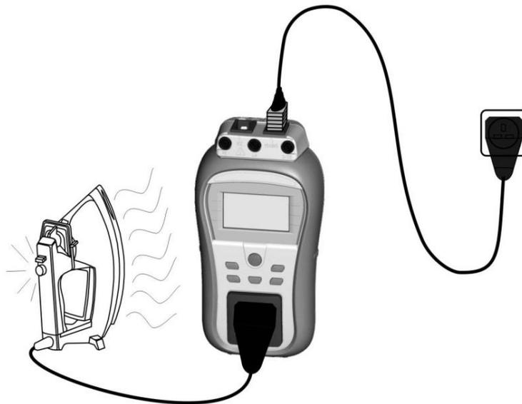
**Figure 5.39:** Power test
