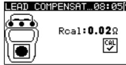
**Figure 4.14:** Lead Compensation screen
