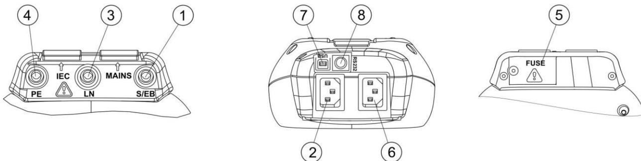
**Figure 2.2:** Connector panel
