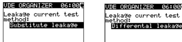
Figure 6.7: Leakage current test method selection screen
