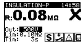
Figure 5.15: Example of insulation resistance - P measurement results
