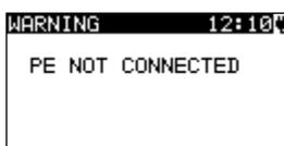
PE between test socket and IEC test terminal is not connected!
