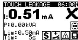
Figure 5.33: Examples of touch leakage current measurement results
