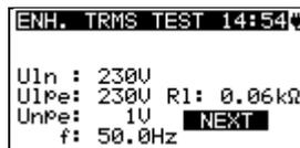
**Figure 6.50:** Enhanced TRMS test result screen
