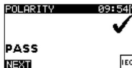
Figure 6.44: Polarity test result screen
