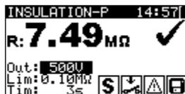
**Figure 6.36:** Insulation resistance - P result screen
