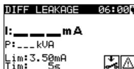
**Figure 6.33:** Differential leakage starting screen
