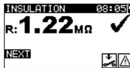
Figure 6.6: VDE Organizer – Insulation resistance result screen
