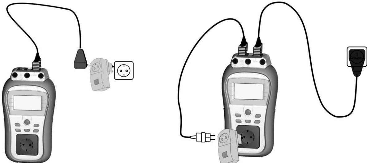
b) Testing of PRCD via mains socket
