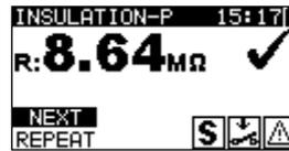
**Figure 6.13:** VDE Organizer – Insulation resistance - P result screen
