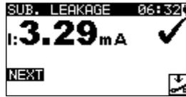
**Figure 6.9:** VDE Organizer – Substitute leakage result screen
