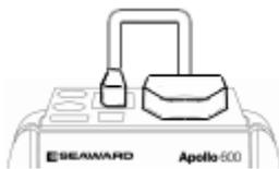
The Polarity test checks the wiring polarity of an IEC lead, the IEC should be plugged into both the EUT and IEC test sockets.
