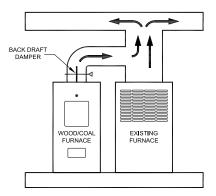
Chimney location is also critical. The furnace must be placed as close as possible to the chimney. You want the chimney connector (smoke pipe) to have a minimum of elbows, two (2) or less. Also, the chimney connector should not have to run more than six (6) feet to the chimney.
