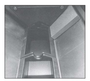
10. Install grate frame (if not already installed): Lay the first grate frame on the side supports and slide to the back of the unit. Then install the second grate frame to the front as shown in the picture above. The smooth ends of the frames should be together in the middle. For the model 30A, insert the half grate frame in the middle of the front and rear frames.
