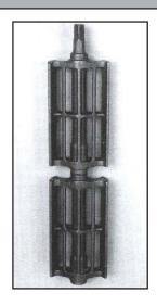
Installing Grates: Install grates together, slip shaker lug into hole and place grates into frame. Grate arch faces upward. Check out grate rotation by placing shaker handle on grate lug (3/4"). Grates should rotate freely.
