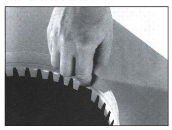
Installing collar to top: To install hot air attaching collar, simply bend all tabs right angle under shroud. This may be possible with thumbs, if not, remove top and use small hammer.
