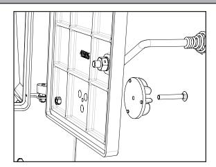
damper up onto the 1/2-13 carriage bolt provided. Then screw the damper and bolt into the door until the bolt protrudes the rear of the door so that a nut can be attached. Tighten the nut.
