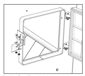
18. Find the Feed Door Latch shown in the parts box. Install with the 1/4-20 bolts and nuts provided. Adjust the latch so that the door seals properly. (The ash door latch shall be assembled in the same manner using the ash door latch.)
