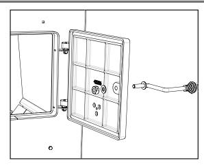
17. To install Feed Door handle, insert handle into the 19. To install the dampers on the doors, screw the door then attach with the 1/2-13 nut and washer provided. Tighten nut against the backside of the door then back it off approx. 1/4 turn or until handle moves freely. (Follow these instructions for ash door handle installation.)
