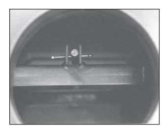
14. Now slip the rear heat plate in behind the rear baffle. Attach heat plate to the firebox by using two (2) 5/16 bolts, nuts & washers. First, line up the top holes and tighten bolts. Secondly, line up the holes in the rear baffle and the heat plate with the firebox and attach by using two (2) 5/16 bolts, nuts & washers. Tighten all four (4) bolts. NOTE: to reach rear bolts you may find it easier to put your arm through the flue outlet rather than to reach through the feed door.
