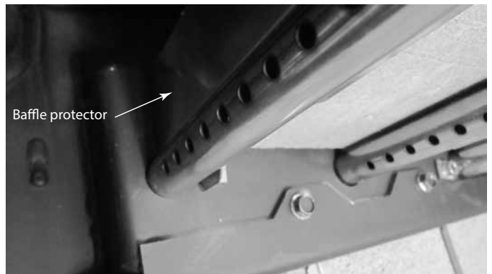
Figure 4.9 Reinstall Baffle Protection Channel
