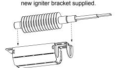
Make sure stud is installed in the proper hole in the igniter cradle.
