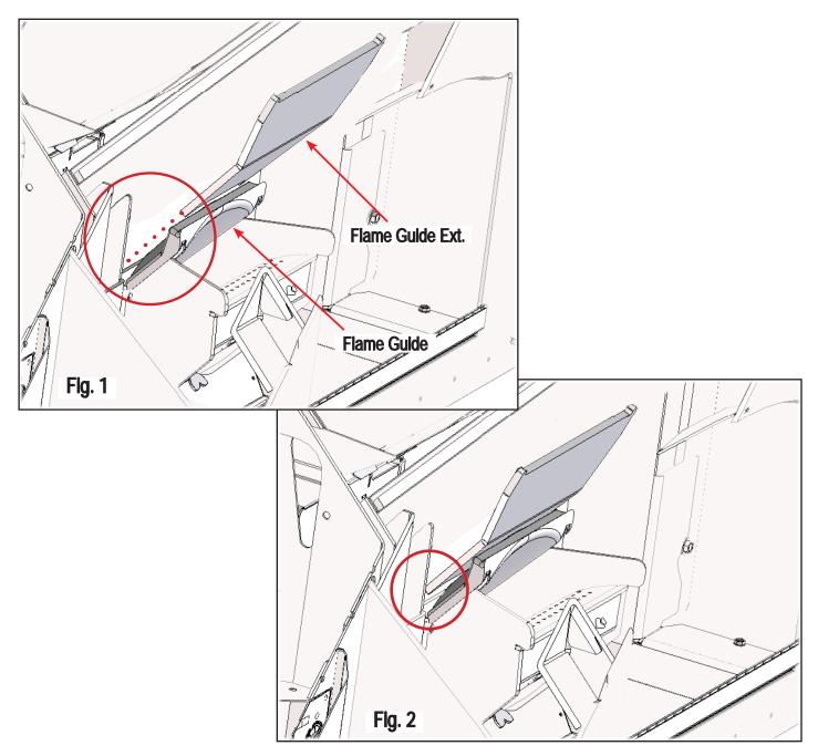
After the flame guide is installed the Flame Guide Extension slides in behind the flame guide as shown in Fig. 1. Make sure Flame Guide Extension is installed the entire way down behind the Flame Guide as shown in Fig. 2.
