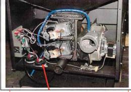
IMPORTANT: Some models are arranged like this and some are slightly different. Be sure to replace the switch closest to the Auger Motors (marked .60" or 1.10"). You will have two switches marked .17" when you are finished.
