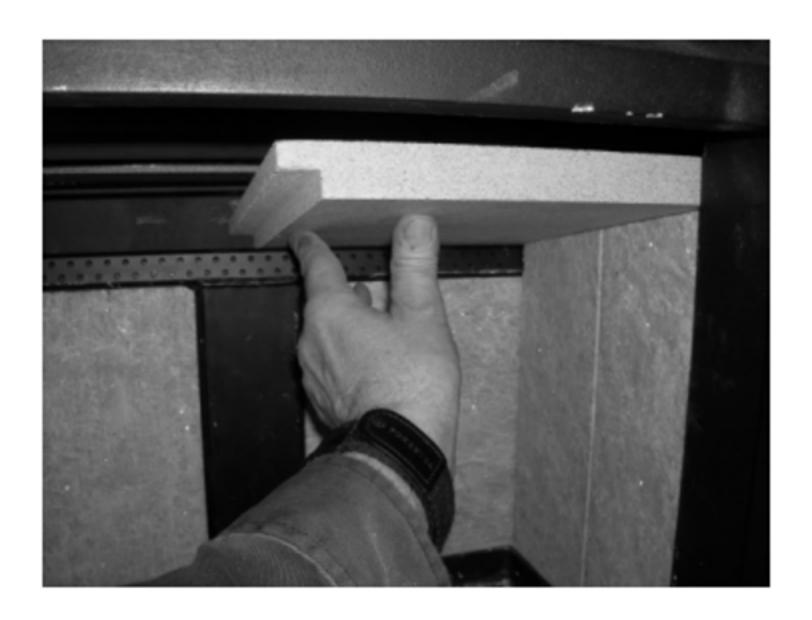
7) While lifting the rear portion of the right baffle, insert the left baffle by engaging the rear and tipping up the front. IMPORTANT – do not force the pieces as they could break or crack – they will fit together without forcing them into place. The two baffles will overlap at the center joint and sit in the grooves of the left and right stones.
