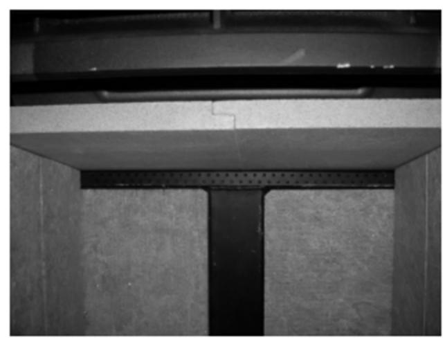
8) Place the baffle guard over the front edge of the baffles. Push it as far back as it will go, onto the baffle plates.
