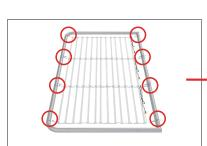
**Step 6:** Connect the feet by inserting into the bottom holes of frame and pressing firmly. Lift frame into upright position.
