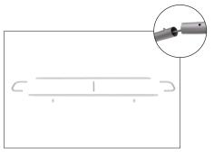
**Step 5:** Zip the edge of graphic beyond the center point as shown to hold the center pole in place. Zip the remaining side and bottom to meet at the corner.
