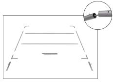
**Step 5:** Unzip print and lay image face up. Slide print onto frame like a pillow case.
