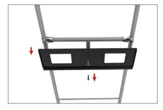
**Step 6:** Attach brackets to back of monitor with screws. Rubber spacers can be placed between the bracket and the monitor if your the back of the monitor is not flat. Choose the spacer that best fits your need. Position the VESA bracket with the hook facing down.
