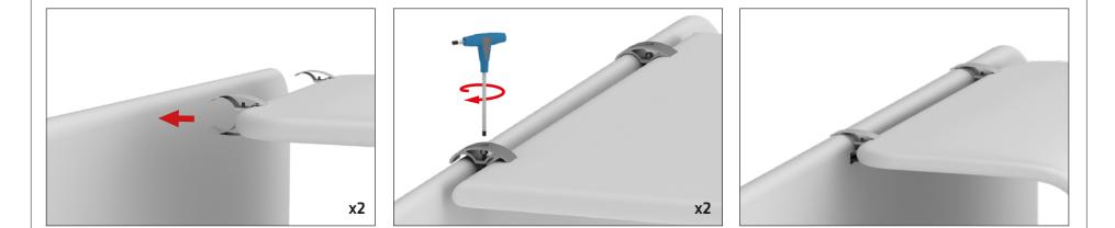
**SHELVING:** Add shelves to frame. Position and level shelves on frame before tightening clamps down with hex tool.
