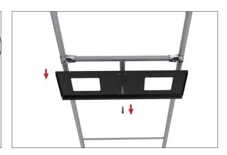
**Step 6:** Intall the hanging brackets onto the back of the monitor. You can also adjust the height of the monitor by moving the position of the brackets up or down using the different holes in the bracket.
