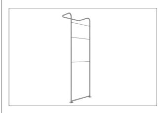
**Step 4:** Fit the fabric over the completed frame. Locate the screw holes on the horizontal clamp bar (for the monitor bracket to mount) and pierce the
