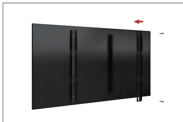
**Step 7:** Hang the monitor onto the waterfall mount and lock into position with set screws.
