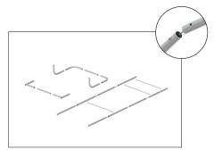
**Step 5:** Insert feet into the holes at the bottom of display.
