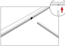
**Step 6:** Add shelves to frame. Position and level shelves on frame before tightening clamps down with hex tool.
