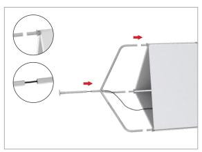
**Step 9:** With wall and hanging sign on their sides, attach hanging sign to center carousel pole using cables and clips. Push tower up into position.
