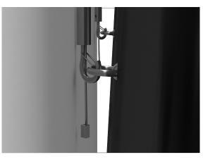
**Step 13:** Thread power cord through bottom grommet and out through bottom of graphic. Zip cable access door closed.
