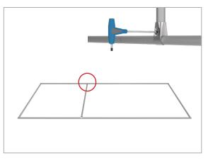
**Step 5:** Install bottom feet by joining two panels together and inserting dual posts into bottom of frame corners. Install connector clips between panels for stability. (x3)
