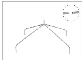
**Step 3:** Install bottom feet by joining two panels together and inserting dual posts into bottom of frame corners. Install connector clips between panels for stability. (x4)
