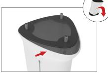
**STORAGE:** The zipper on the back is used to access storage. **Step 3:** Place counter top onto poles. Tap down with hand until top rests securely on push buttons and the top of the poles stick out.
