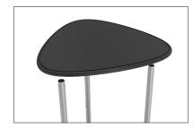
**Step 7:** Tap down base with hand to secure. Turn counter back over.
