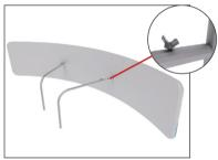
15. Slide the hanging post on to on to the small shaft.
