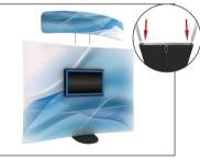
16. Lift header and place on top the header and tighten the bolts of the frame that is holding the TV unit.
