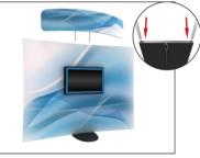
16. Lift header and place on top the header and tighten the bolts of the frame that is holding the TV unit.
