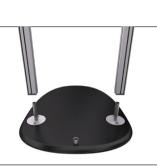
Lift the frame and fit to the base, push it all the way in to the round plate.
