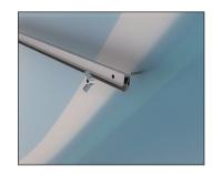
8. From the back insert the 2 bolts that secure the TV profile. There are 3 holes you can select the height you need, push the fabric against the screw and make a hole in the fabric.
