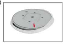
**Step 6:** Zip the two edges of graphic to the center point as shown.
